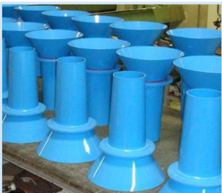
Funnels from Volta material
